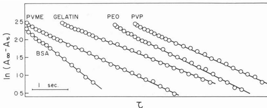
FIGURE 1. Plots of  $\ln(A_\infty - A_\tau)$  against  $\tau$ .  $A_\infty$  is the initial amplitude of the free induction decay signal following the  $90^\circ$  pulse at time  $\tau$ .  $A_\tau$  is  $A_\tau$  as  $\tau \rightarrow \infty$ . The data illustrate that the plots can be fitted with a single slope, equal to  $-(T_1)^{-1}$ . The concentrations were: BSA (10.0%); gelatin (2.94%); PVP (5.66%); PEO (7.67%); PVME (8.6%).
