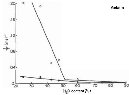
FIGURE 6. Plots of  $(T_1)^{-1}$  ( $\bullet$ ) and  $(T_2)^{-1}$  ( $\circ$ ) against the water contents of different concentrations of gelatin gel. Data same as in Figure 4.
