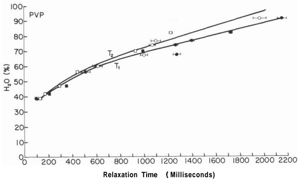
FIGURE 7.  $T_1$  and  $T_2$  water protons in aqueous solutions of polyvinylpyrrolidone (PVP) against their water contents.
