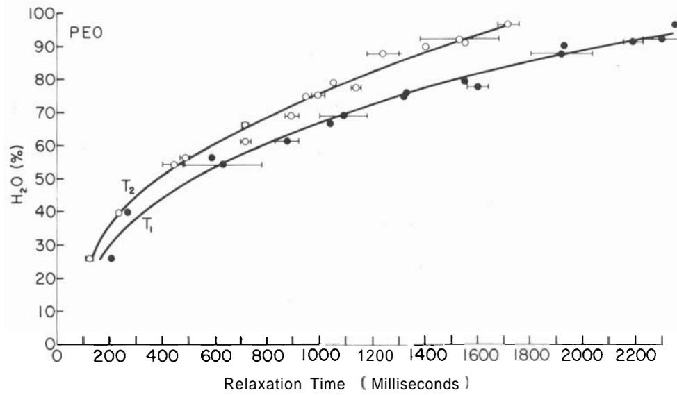
FIGURE 8.  $T_1$  and  $T_2$  of water proton in aqueous solutions of poly(ethylene oxide) (PEO) against their water contents.
