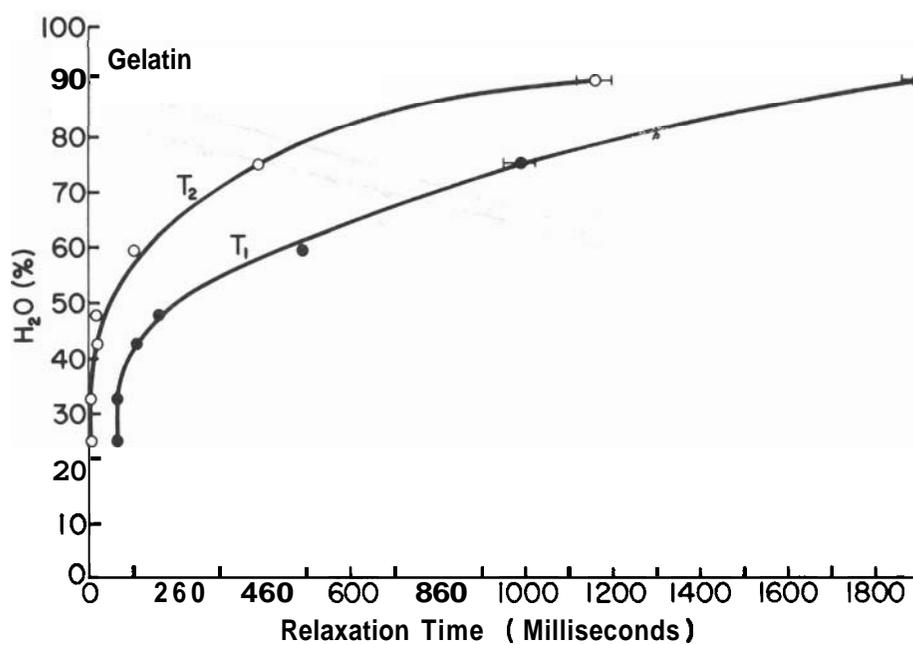
FIGURE 4.  $T_1$  and  $T_2$  of water proton in aqueous gelatin gel plotted against their water contents.
