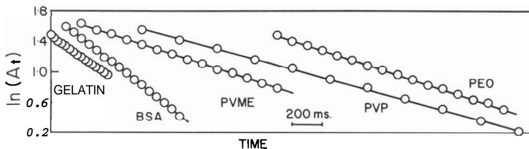
FIGURE 2. Carr-Purcell plots of  $\ln A_t$  against  $t$  where  $A_t$  is the echo height at time  $t$ . The data illustrate that the plots can be fitted with a single slope equal to  $-(T_2)^{-1}$ . The concentrations were: BSA (8.3%); gelatin (8.0%); PVP (9.3%); PEO (6.1%); PVME (9.9%).
