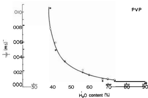
FIGURE 10. Plots of  $(T_1)^{-1}$  (●) and  $(T_2)^{-1}$  (○) against the water contents of the solutions of polyvinylpyrrolidone of different concentrations. Data same as Figure 7.
