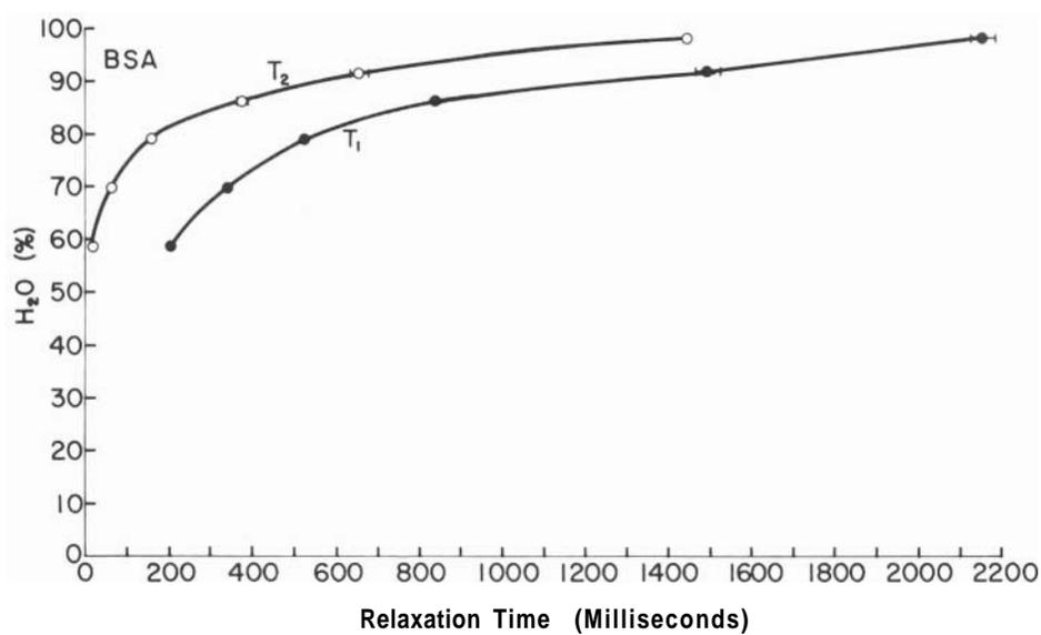
FIGURE 3.  $T_1$  and  $T_2$  of water proton in aqueous solutions of bovine serum albumin plotted against their water contents.
