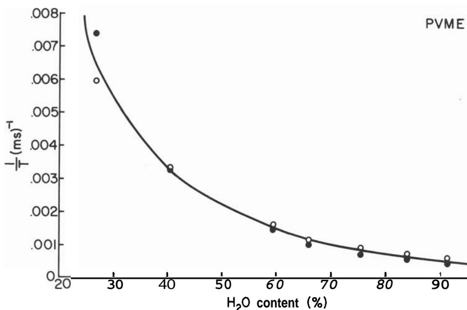
FIGURE 12. Plots of  $(T_1)^{-1}$  (●) and  $(T_2)^{-1}$  (○) against the water contents of various polyvinylmethylether solutions. Data same as in Figure 9.
