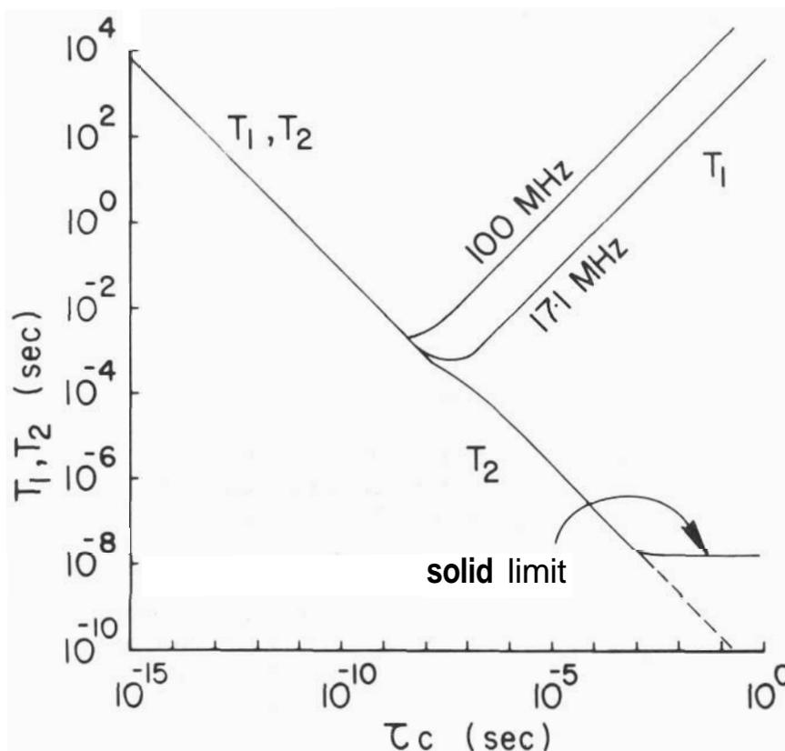
FIGURE 13. Theoretical curves of  $T_1$  and  $T_2$  of water proton at various rotational correlation times,  $\tau_c$ , calculated from the equations of Bloembergen, Purcell and Pound (1948) as modified by Kubo and Tomita (1959):
