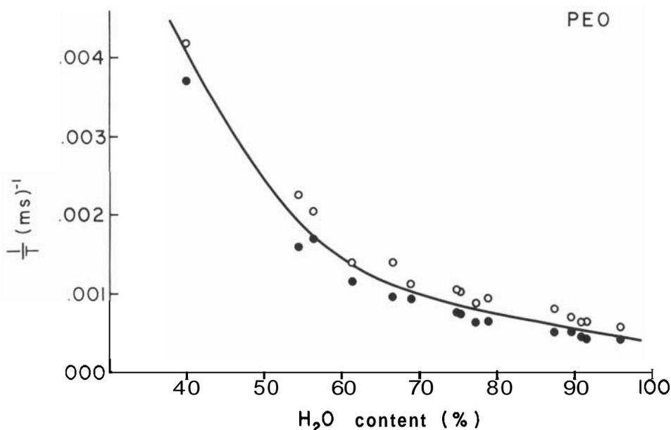
FIGURE 11. Plots of  $(T_1)^{-1}$  (●) and  $(T_2)^{-1}$  (○) against the water contents of poly(ethylene oxide). Data same as in Figure 8.
