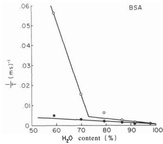
FIGURE 5. Plots of  $(T_1)^{-1}$  ( $\bullet$ ) and  $(T_2)^{-1}$  ( $\circ$ ) against the water contents of different concentrations of bovine serum albumin (BSA). Data same as in Figure 3.
