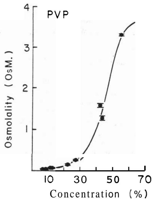
FIGURE 2. Osmolality of polyvinylpyrrolidone (PVP) solution at varying concentrations. Details are the same as in Figure 1.
