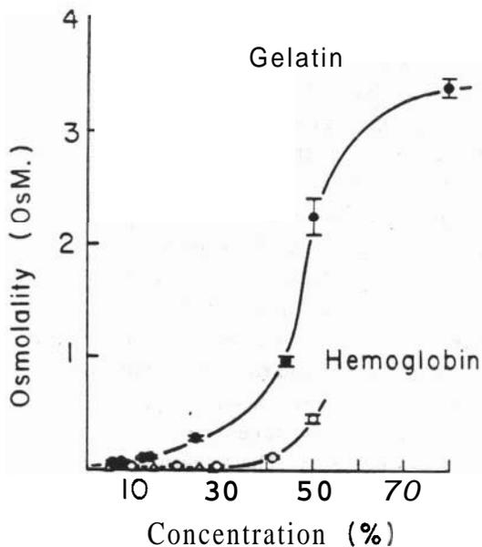
FIGURE 1. Osmolality of gelatin and hemoglobin at varying concentrations. Osmolality is given in Osmolal concentration. Protein concentrations are in % (wt wt). Each point is the average of at least 4 independent determinations and the distance between horizontal bars are twice the standard errors. Six extra points on the hemoglobin curves shown as A's are taken from Adair's data (see text).
