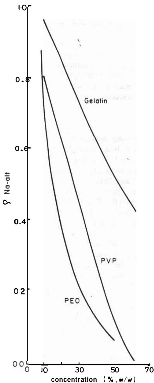
FIGURE 6. Plots of apparent equilibrium distribution coefficients of Na<sup>+</sup> salts (p-value) of polymer water system against polymer concentration given as % (w/w). (from Ling and Ochsenfeld<sup>40</sup>).
