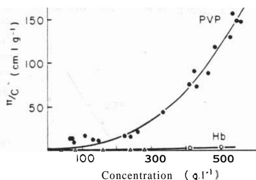
FIGURE 4. Plot of  $\pi/C$  against  $C$  in PVP solutions. Osmotic pressure,  $\pi$ , is in units of cm of  $H_2O$ : $C$  in grams of polymer per liter. Data are the same as in Figure 2, except that standard error bars are not represented. The solid line going through the experimental points are based on Equation I. Values of virial coefficients chosen to fit the data are given in Table I. For comparison the hemoglobin data of our own and from Adair are also shown.
