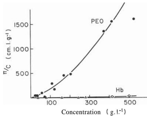
FIGURE B.  $\pi/C$  vs.  $C$  plots of PEO solutions. Details are similar to those described in Figure 4. Value of **virial** coefficients are those given in Table I. For comparison hemoglobin data of our own and from **Adair** are also shown (from Ling, 1984).
